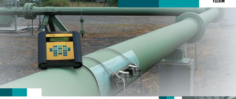
FLEXIM's range of FLUXUS<sup>®</sup> G60X portable gas flow meters not only covers virtually any gaseous medium, they also include all liquid flow metering capabilities of the FLUXUS<sup>®</sup> F60X series meter series making them a truly comprehensive tool.
